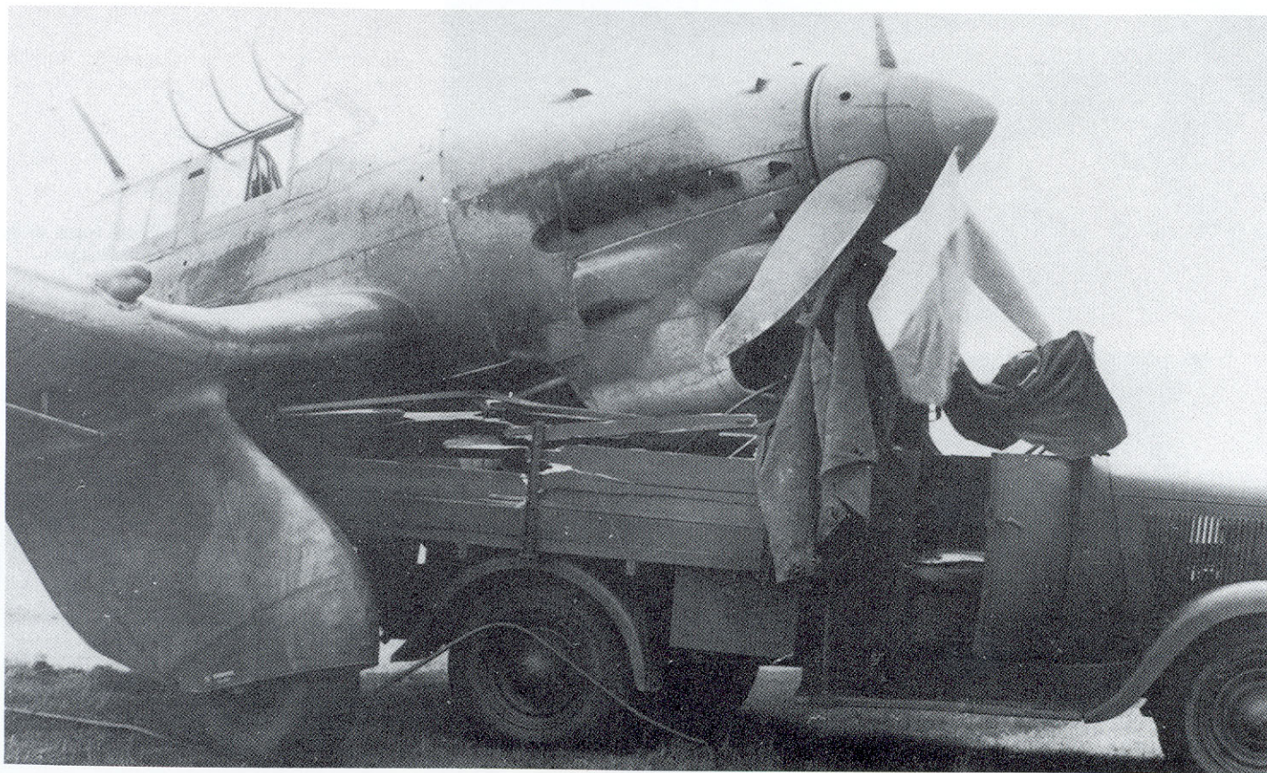
This ground collision between a Ju 87 A-2 and an unfortunate truck was the result of brake failure.
